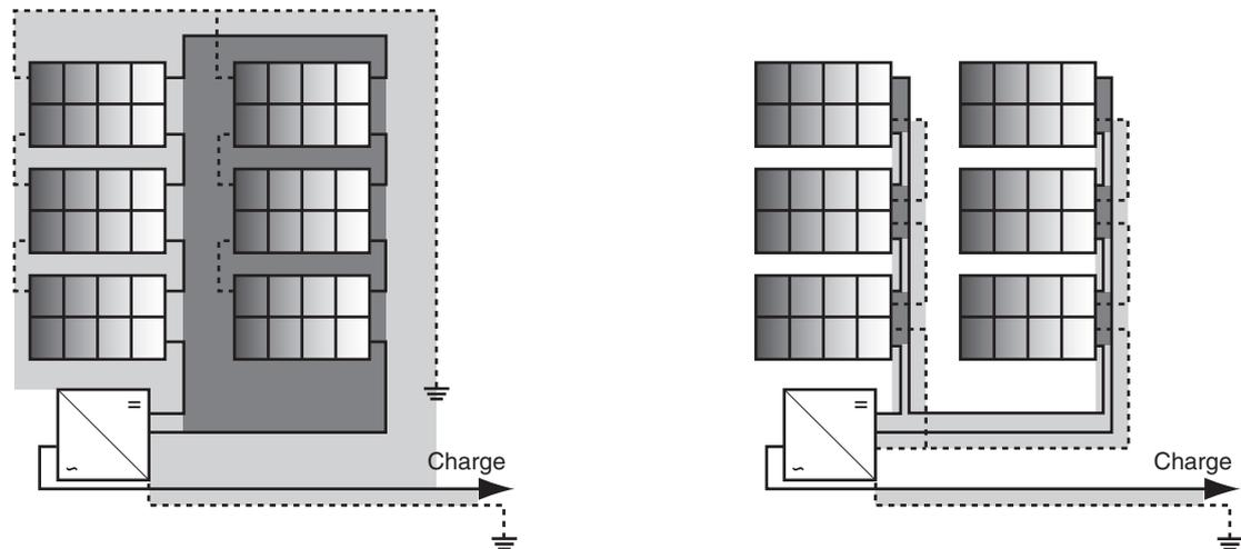
Fig. P13 : Avoiding loops when cabling strings
